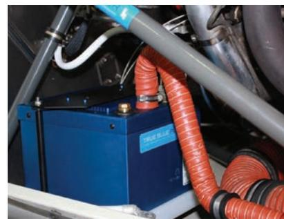
Installation of TB17 Certified Lithium-ion Battery in Robinson R44
