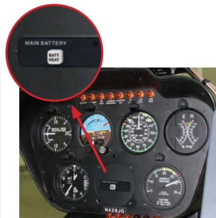
The MD41-1817 ACU combines the necessary battery annunciations and heater control required for proper pilot interface to the battery system
